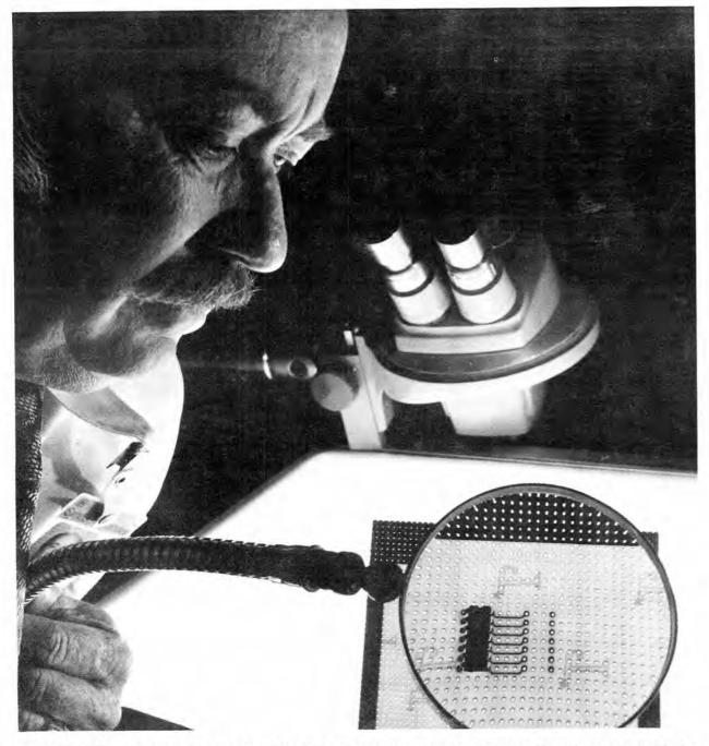
PREPUNCHED printed circuit board fabricated by a new technique which eliminates drilling "through-holes" in the dielectric substrate is examined by inventor T.A. Aller, 7123-1. The magnified section of the photo shows an integrated circuit (rectangle) with copper-clad circuitry and plated through-holes to its right.
